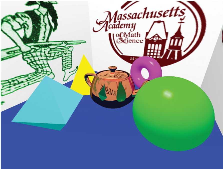
COLOR PLATE 25 Render to texture with FBOs to improve performance of dynamic environment mapping. (For Figure 18.5 in Chapter 18)
