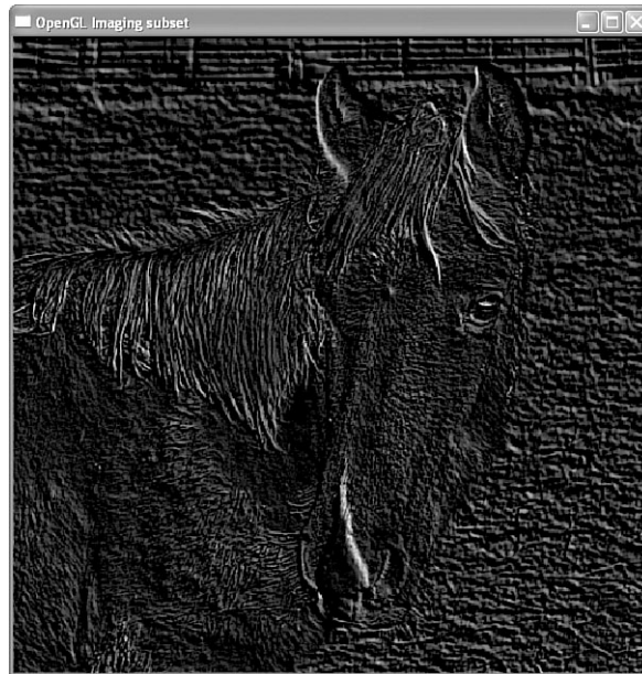
FIGURE 7.13 Using convolutions and the color matrix for an embossed effect.
