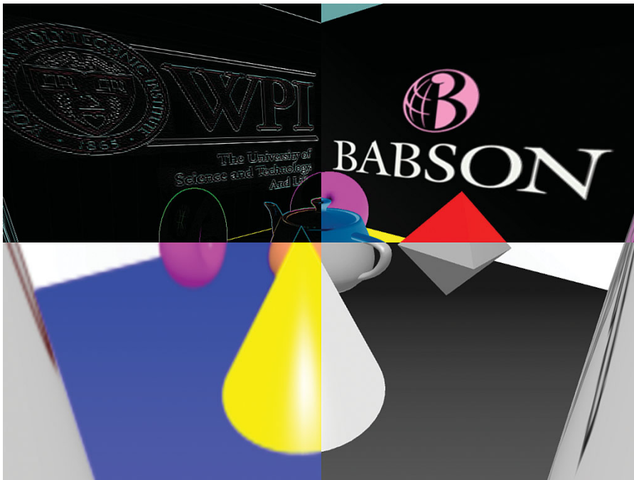
COLOR PLATE 26 Fragment shaders can simultaneously output multiple distinct colors to separate color buffers attached to FBOs. (For Figure 18.6 in Chapter 18)
