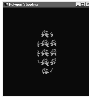
FIGURE 3.30 PSTIPPLE output with the polygon rotated, showing that the stipple pattern is not rotated.
